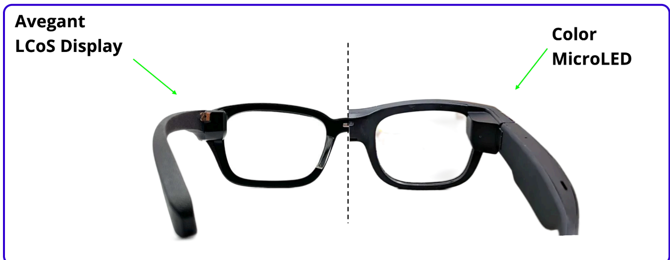
Figure 12, Comparison of Avegant AG-30L2 (left) versus JBD Hummingbird I (right) shown on Rayneo X3 Pro - [3]
