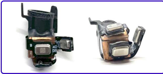
Figure 10, Images of the JBD Hummingbird I (from Rayneo X2) with its heat sinks and demura memory-[3]
